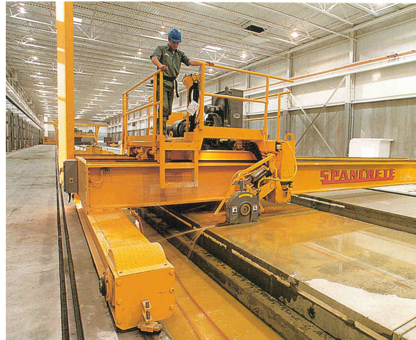
Cutting PARTEK hollow core slab
