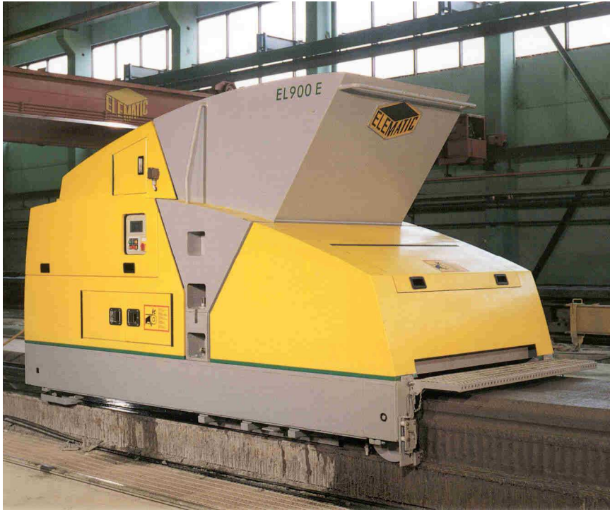
Casting PARTEK hollow core slab
