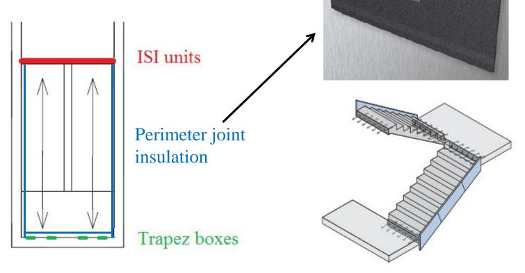
The type and number of supporting elements should be specified in the structural analysis according to the values of reactions (not required in the homework)
