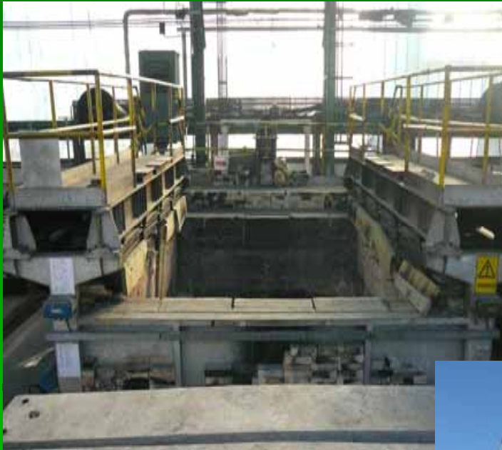
Horizontal testing furnace
