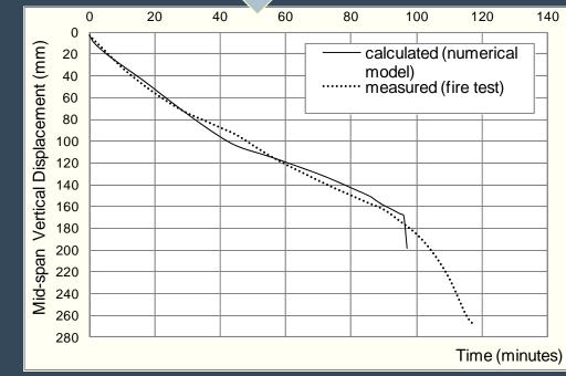
2. <u>Thermo-mechanical modeling of composite slabs with thin-</u> walled steel sheeting submitted to fire
