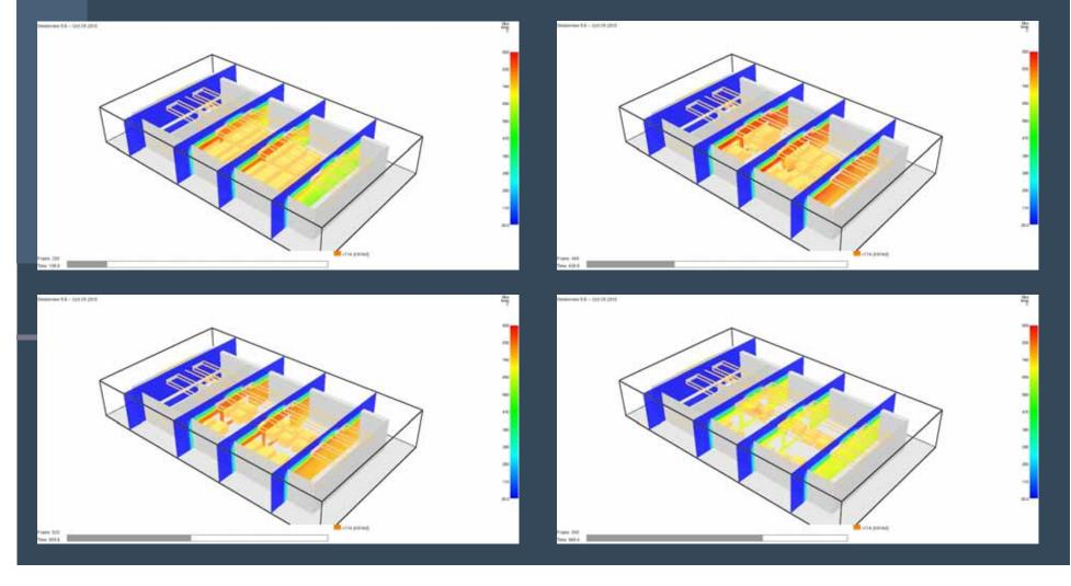
**1. Numerical simulation of the natural fire event in an industrial building using FDS**
