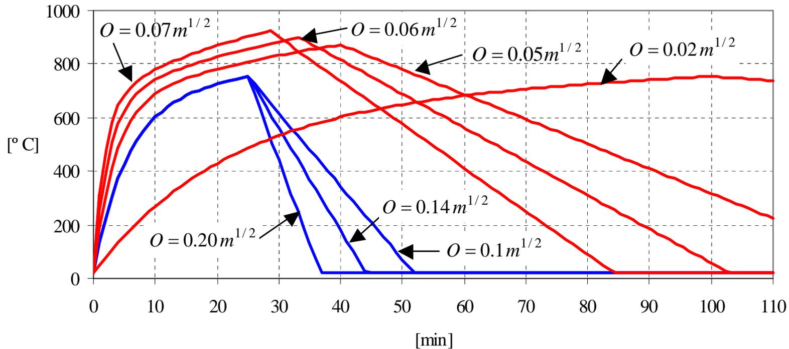
— Ventilation controlled fires      — Fuel controlled fires
