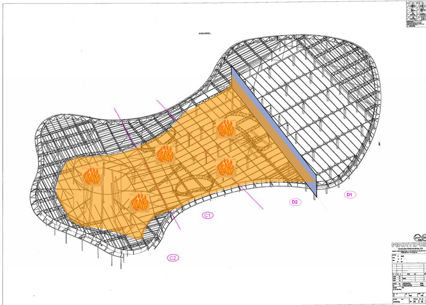
It was assumed that the fire would developed in all the 3 parts D2, C1 and C2.
