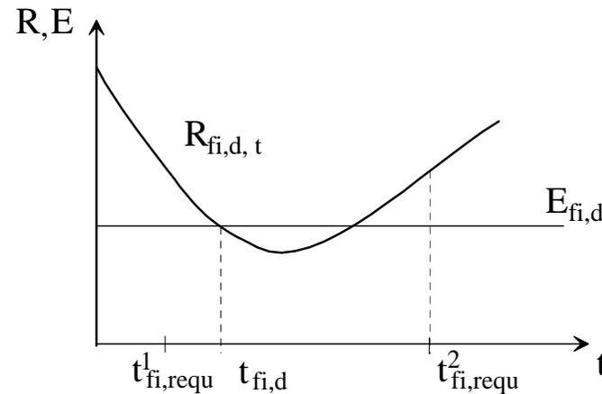
Collapse is prevented during a required period of time,  $t_{fi,requ}^1$
