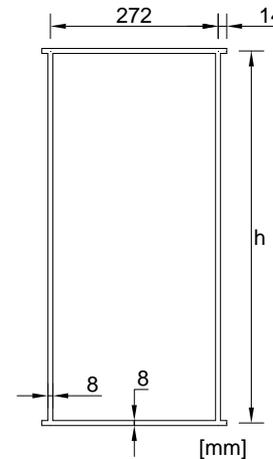
Note: In a prescriptive approach and without making any calculation, this structure should have been protected for a critical temperature of 350°C and for R60
