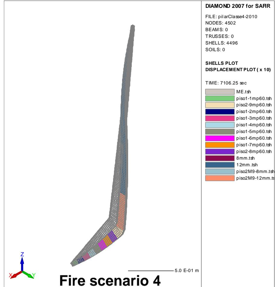
Without protection - collapse at 14 min
