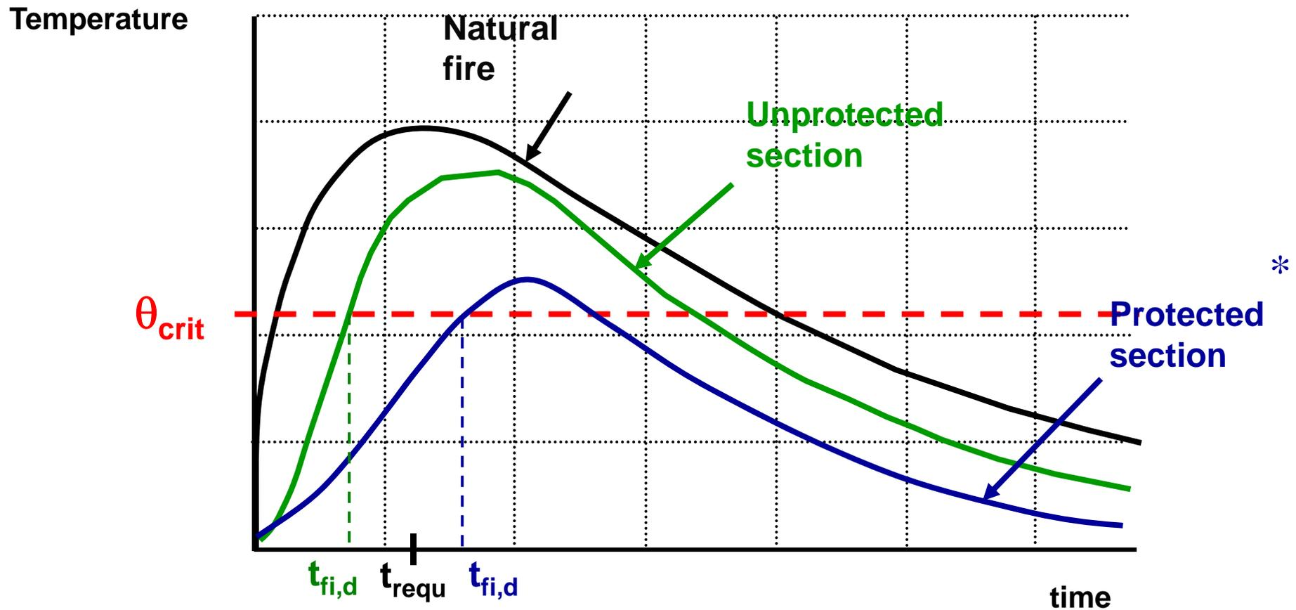
$$t_{requ} \leq t_{fi,d} \quad !$$
