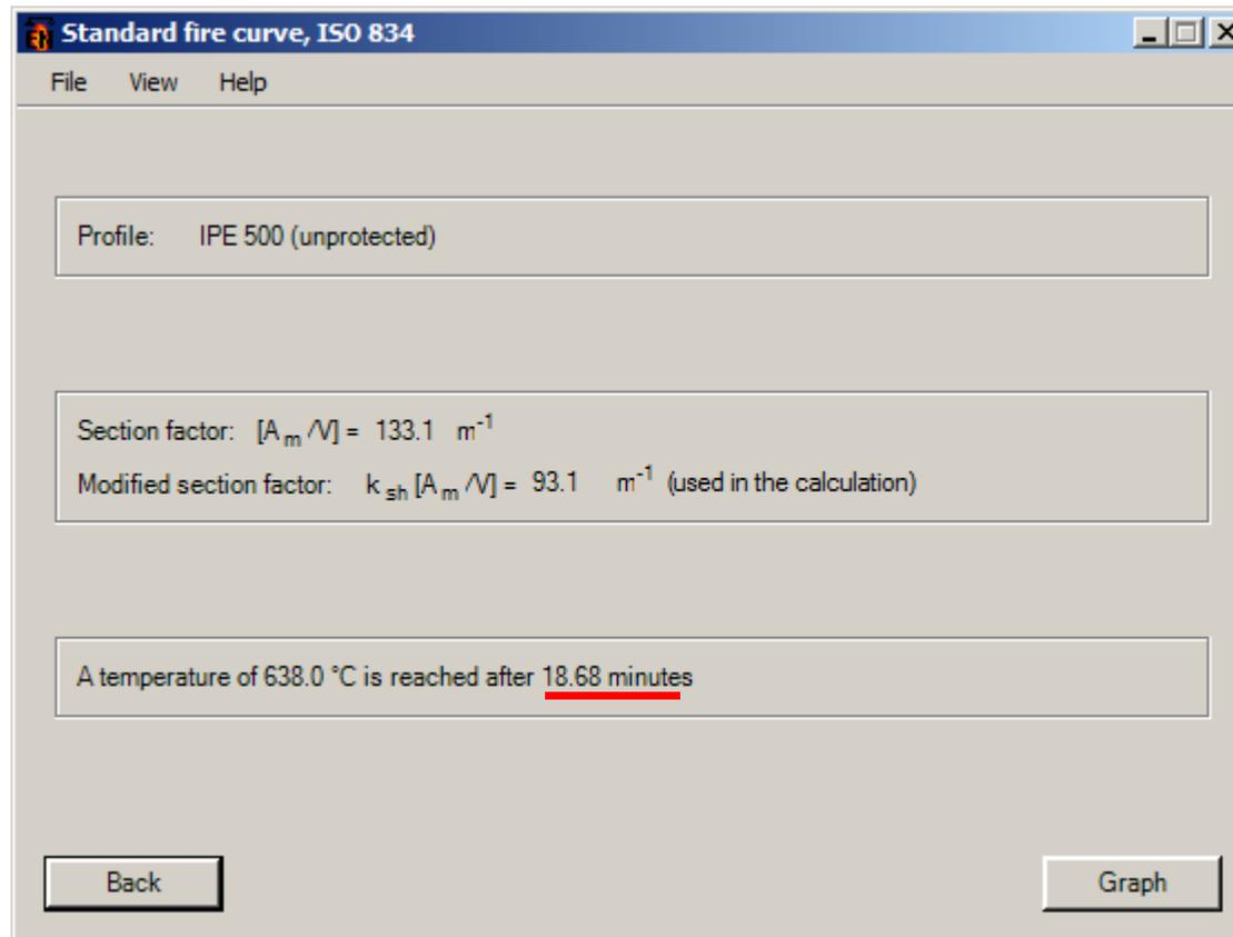
$t_{fi,d} < t_{requ} = 60 \text{ min} \Rightarrow$  Fire protection is needed for a critical temperature of  $\theta_{a,cr} = 638 \text{ °C}$
