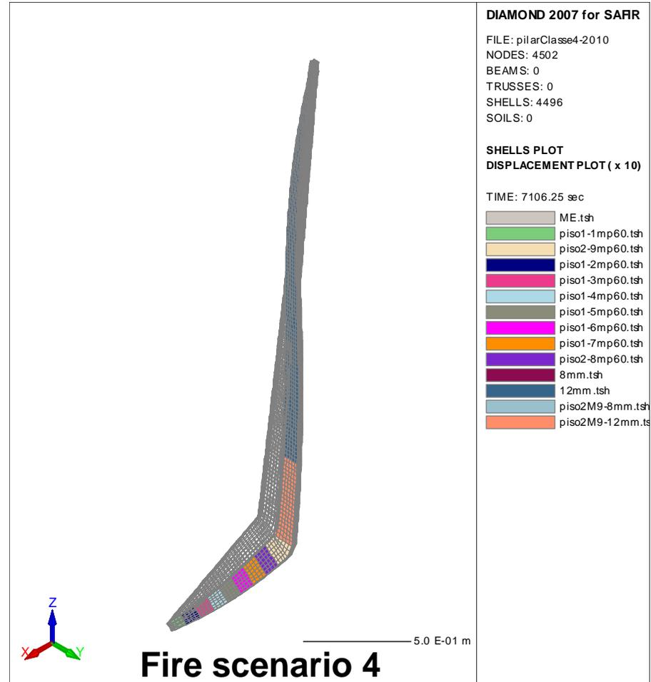
Without protection - collapse at 14 min
