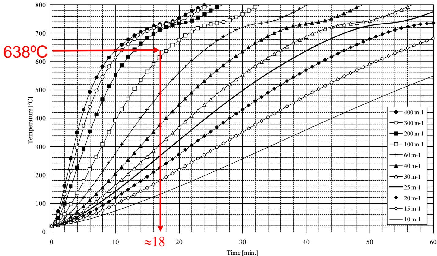
$t_{fi,d} < t_{requ} = 60 \text{ min} \Rightarrow$  Fire protection is needed for a critical temperature of  $\theta_{a,cr} = 638 \text{ }^\circ\text{C}$
