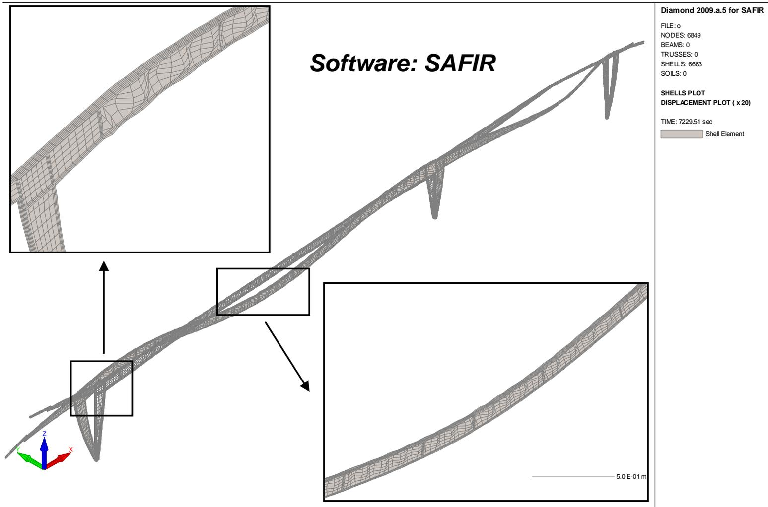
Deformed shape at Zone A, for the combination of actions 1, after 120 minutes (x20)
