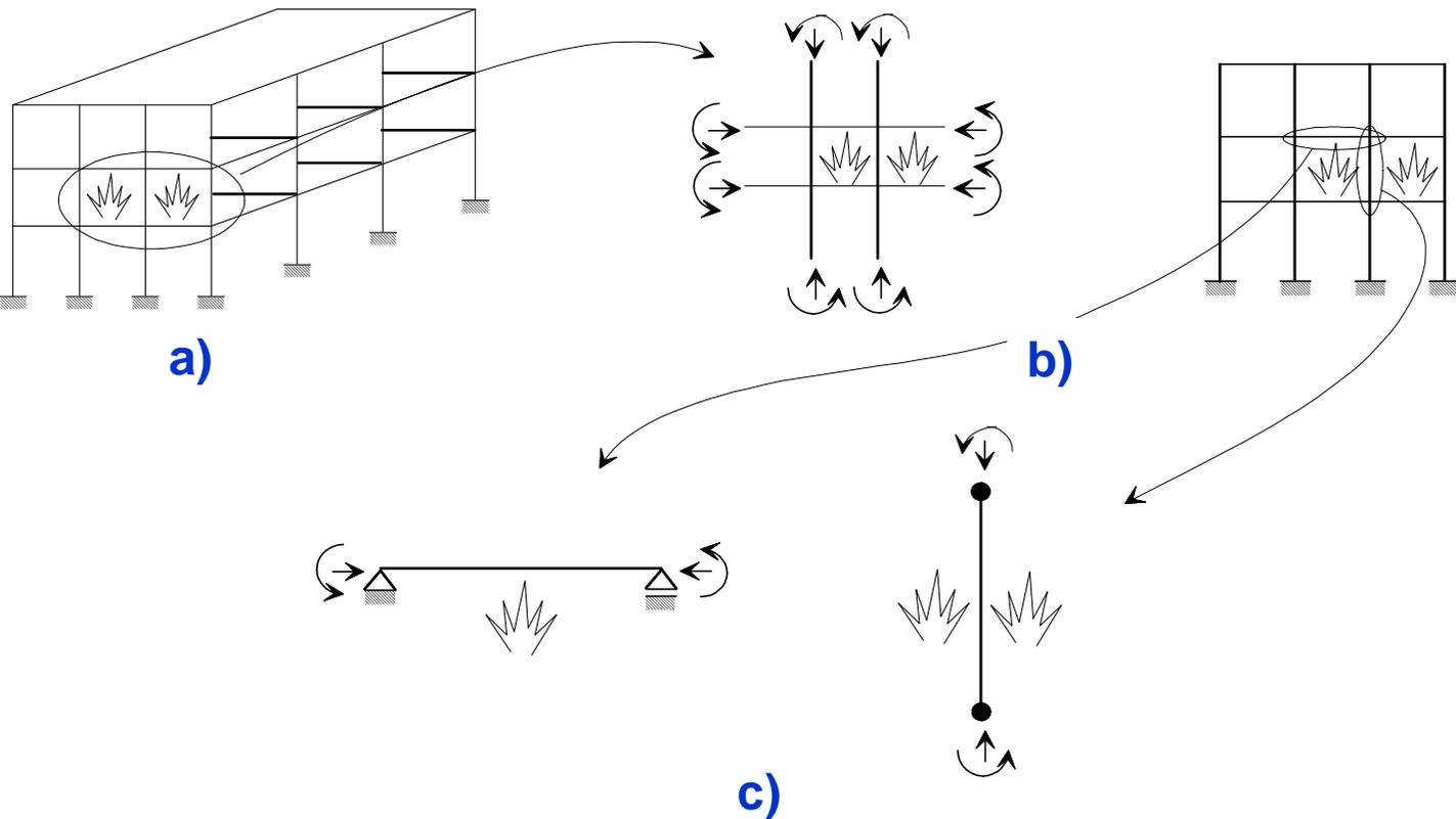
**Analysis of: a) Global structure; b) Parts of the structure; c) Members**
