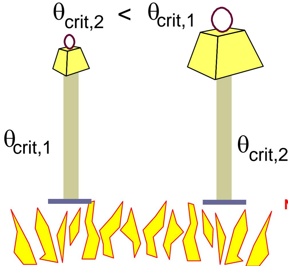
The designer should provide the owner with value of the critical temperature, so that the thickness of the fire protection material can be defined in a more economical way.
