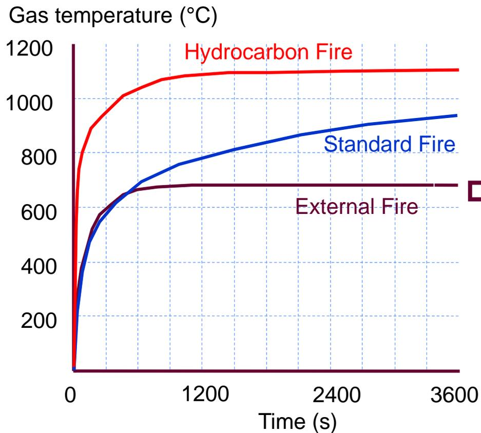
EC3 and EC9 do not use this external fire curve. A special Annex B on both Eurocodes gives a method for evaluating the heat transfer to external steelwork
