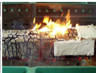
Multiple shear steel-to-timber dowelled connection
