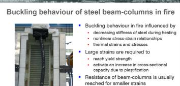
Buckling of a SHS section at elevated temperature
