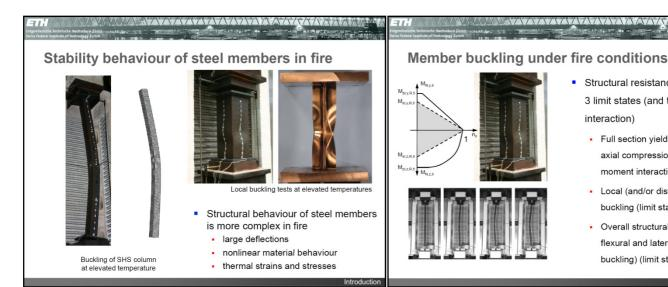
Local (and/or distorsional) buckling (limit state 2)
