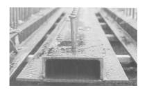
Investigation in the behaviour of continuous slim floor beams at room temperature and in fire
