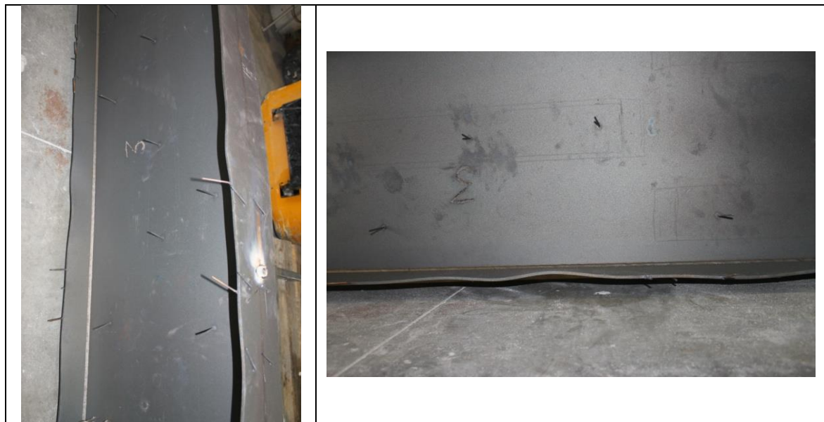
Figure 102: Deformed shape after test 3
