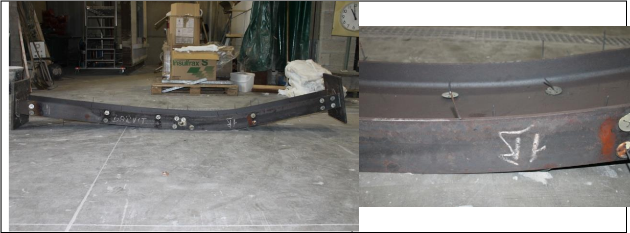
Figure 98: Deformed shape after test 1
