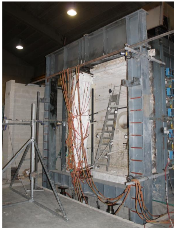
Figure 92: Testing frame for the experimental tests with the equipped column
