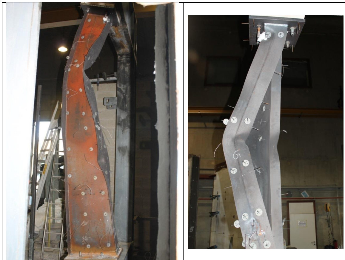
Figure 104: Deformed shape after test 4
