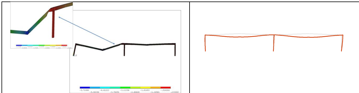
Figure 155: Failure mode for internal column fire: left) shell model, right) new beam element model
