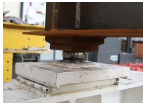
Figure 55: Pinned point supports: a) fixed; b) free
