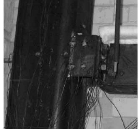
Figure 3: The reverse channel joint tested
