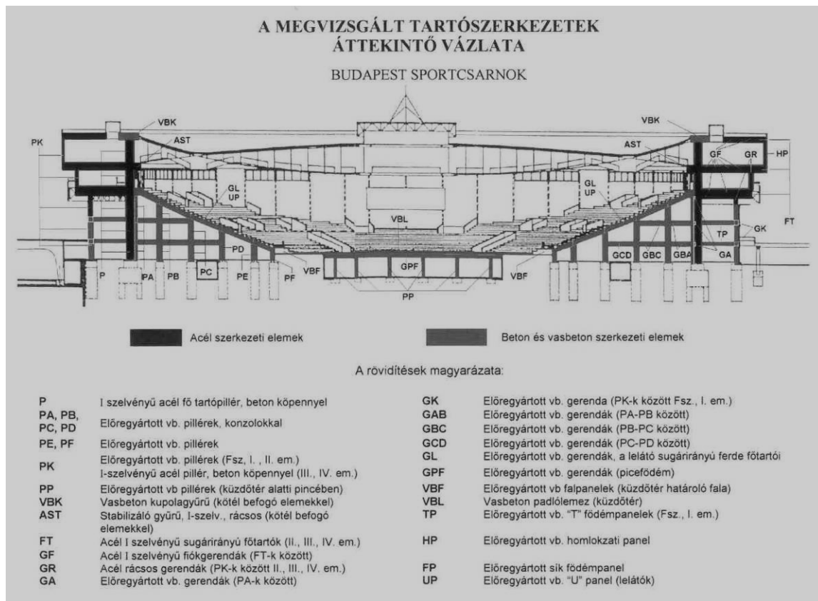
Figure 3.1.1 The structure of the Budapest sport stadium.
