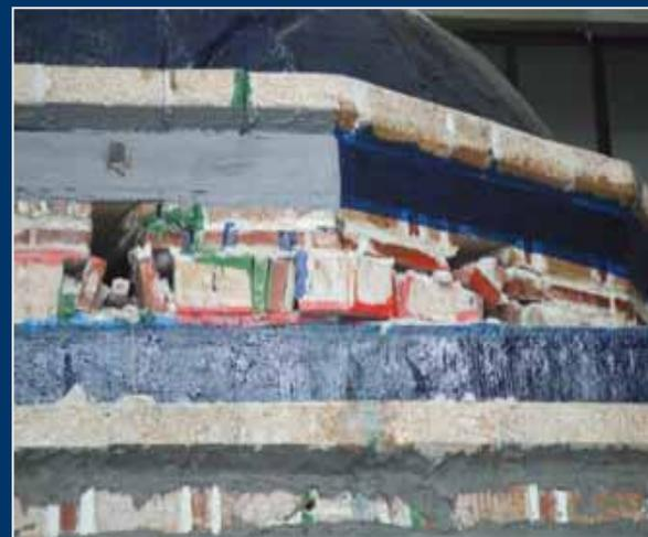
Heavy damage on many parts of the model was observed: many cracks developed on the dome and on the walls around the openings. Due to the intensive shaking inclination of one corner of the model occurred and at that part damage at the FRP belt developed.
