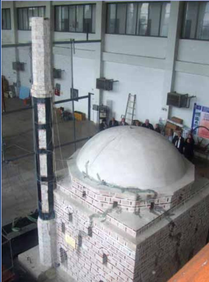
*Such a strengthening enabled stiffening of the minaret and increasing of its bending resistance*
