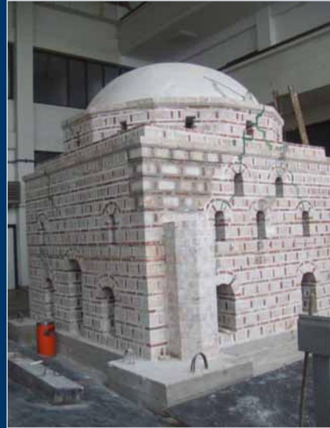
Rebuilding of the damaged part after phase 2 testing
