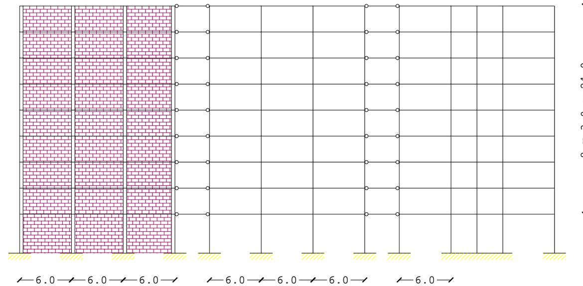
9-Storey dual R/C building with masonry infills
