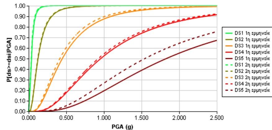
high-rise frame structures, regularly-infilled, designed to High code (NEAK/EAK2000)
