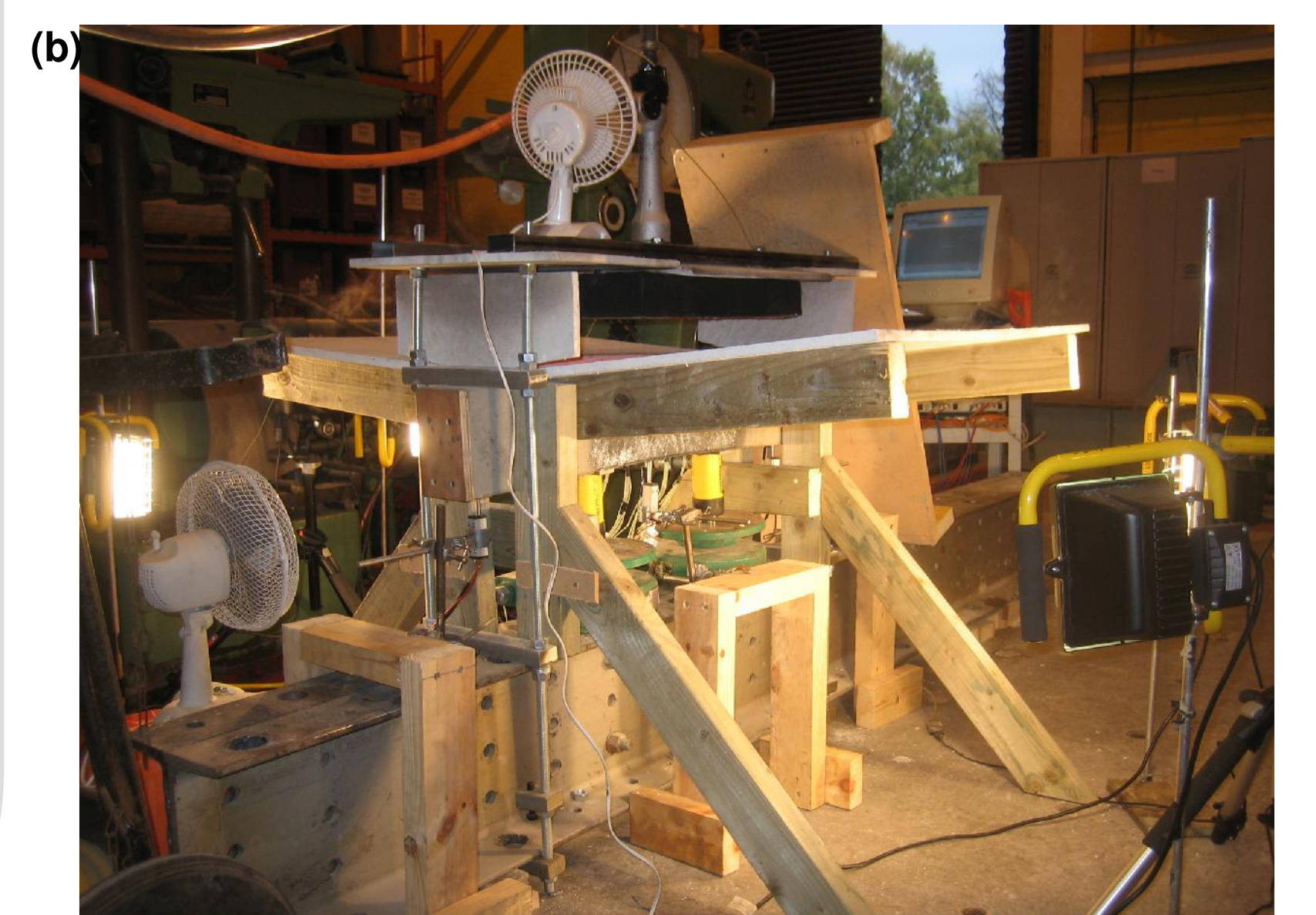
Figure 1 – (a) Mechanical control showing crack pattern of beam at ultimate load. (b) Thermal testing of tensile cracked section in progress
