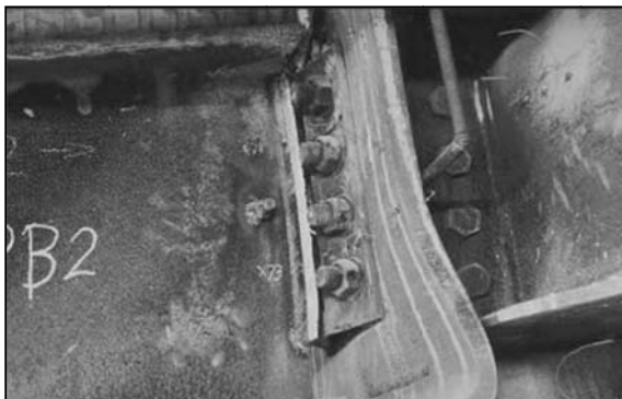
Fig. 1 Fracture of a Partial depth endplate connection
