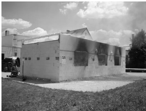
Fig. 1 First Munich fire test
