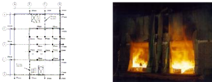
Fig. 2. Fire test of a full-scale reinforced concrete building, 2001 (BRE) Cardington [6]
