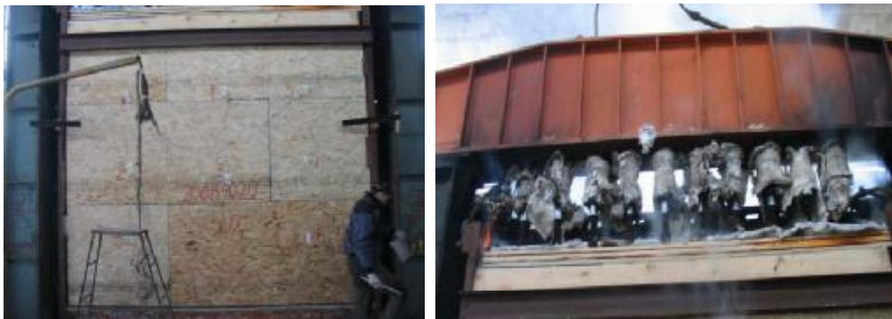
Figure 3 Locations of thermocouples
