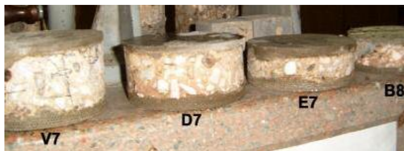
Fig. 6. Deteriorated concrete specimens, prepared for testing
