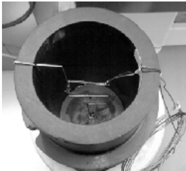
Fig.2 Thermocouple and formwork
