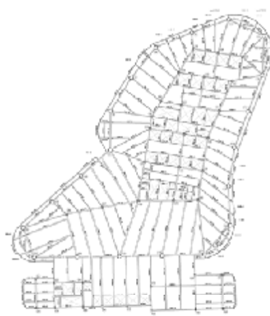
Fig 2 : Typical beam layout for lower floor (Floor 5)
