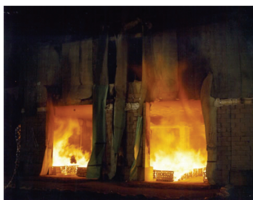
2001 Fire Test on the Full-Scale, Seven-Storey, Concrete Building (BRE) Cardington
