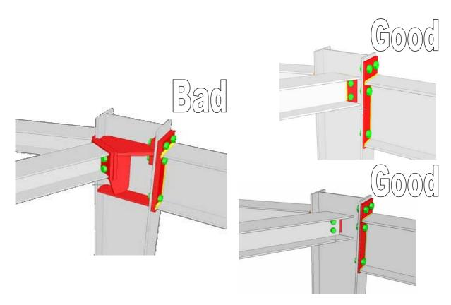
Figure 13.5 Beam to column joint with moment connection to major axis and simple connection to minor axis, unsuccessful case because of unclear transfer of forces, an expensive solution; secondary beams HE120A; moment connection: beam IPE270; bolts 6xM16
