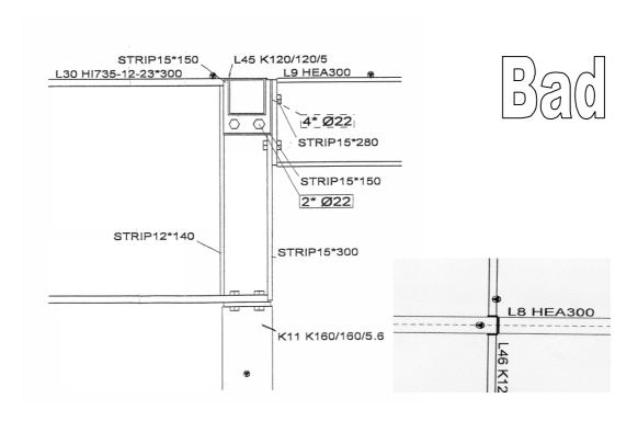
Figure 13.9 Simple beam to column joint, beams of open cross sections, column RHS tube; unsuccessful case - danger of instability during erection and an expensive solution
