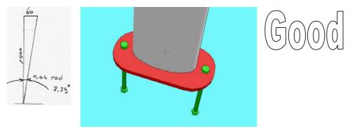
Figure 13.12 Base plate, successful case with simple base plate, in global analyses the stiffness can be introduced
