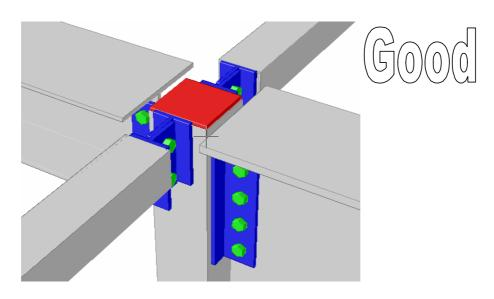
Figure 13.10 Simple beam to column joint, successful case by web angles
