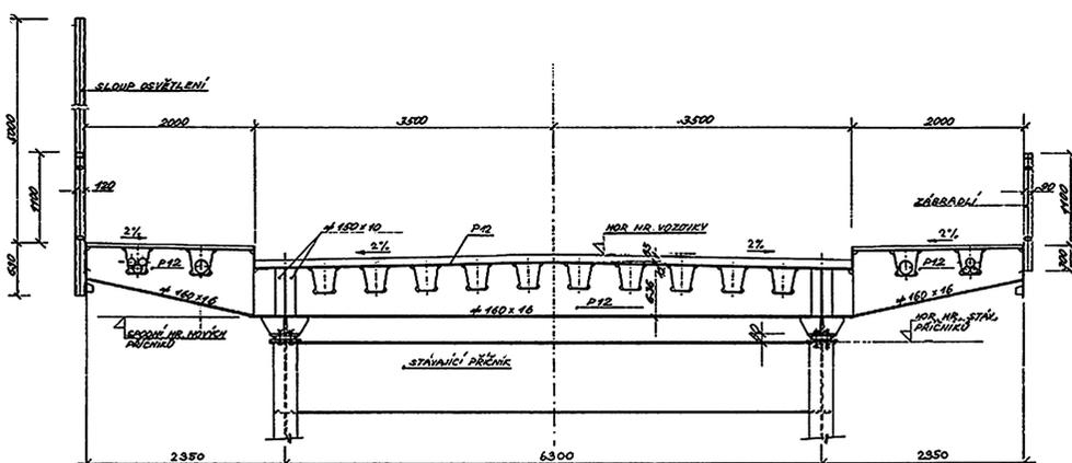
Original drawings: Cross section through an orthotropic bridge deck
