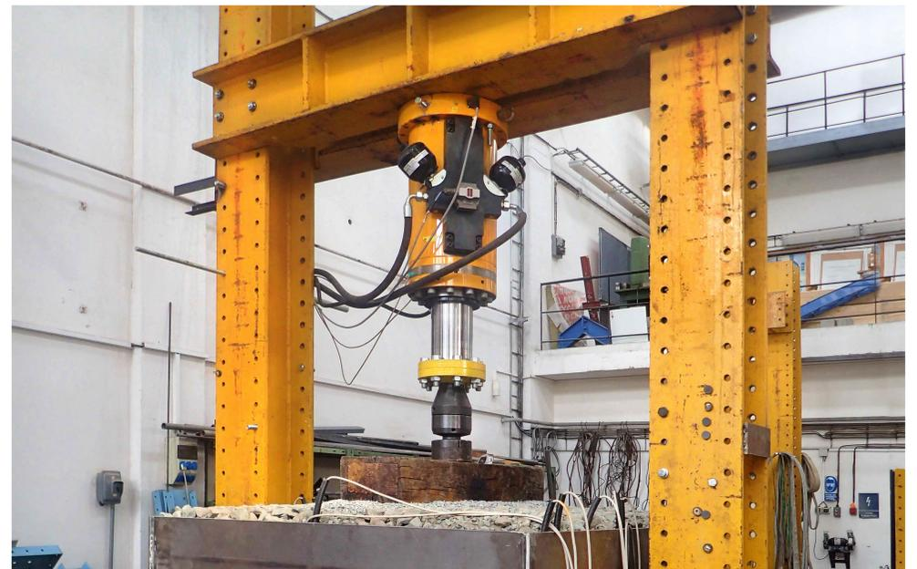
Test assembly with gravel bed and sleeper
