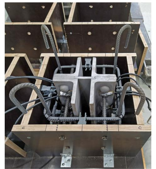
Specimen for pilot test samples before concreting
