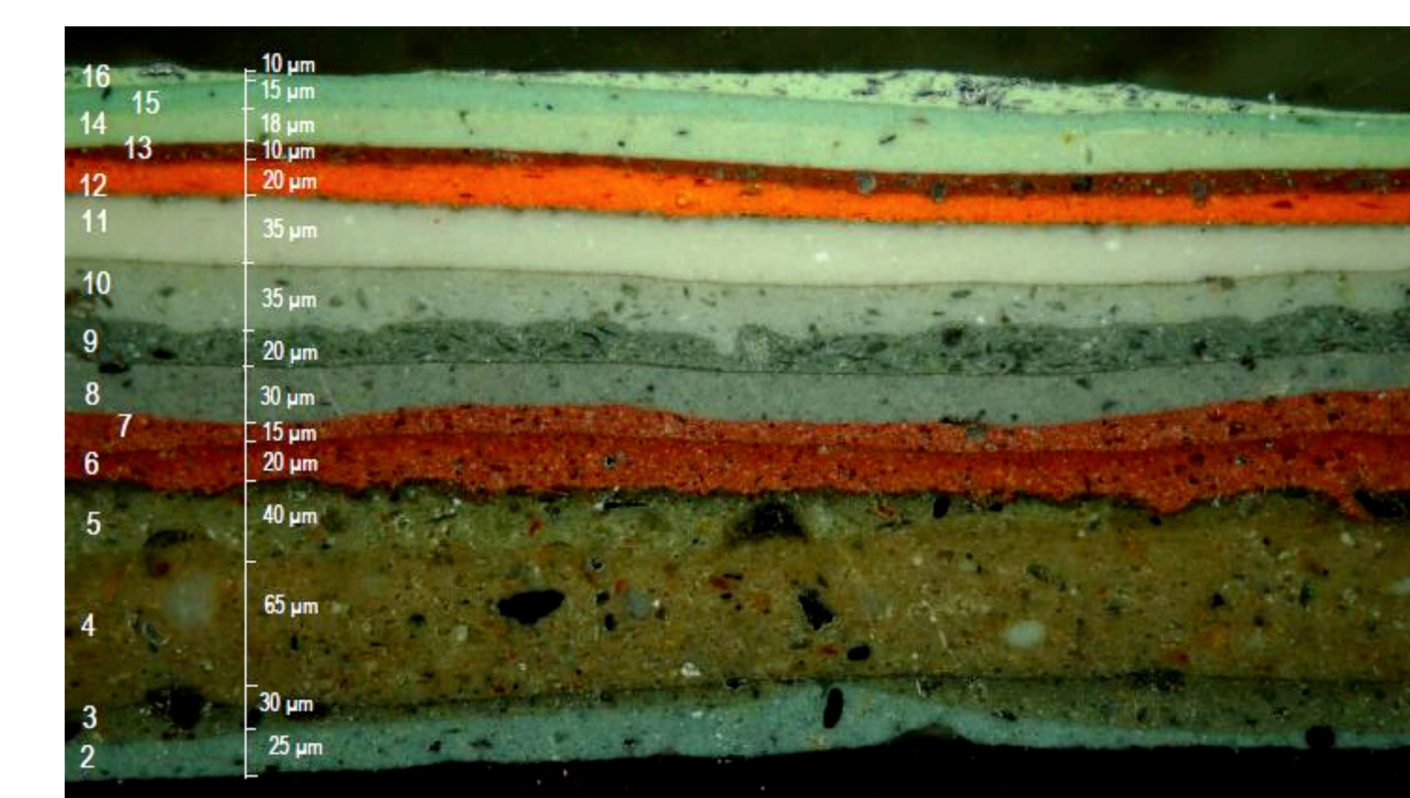
Duplex system – measurement of thicknesses of individual layers
