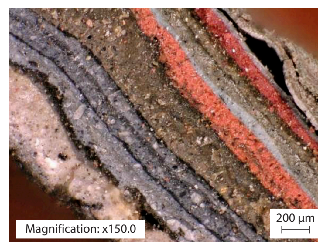
Duplex system – measurement of thicknesses of individual layers
