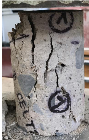
Figure 3.1-2 - Concrete core from abutment (MP-6) after compression test
