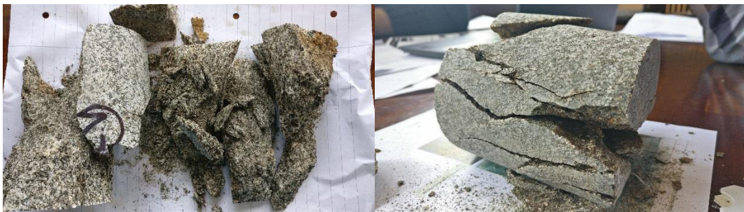
Fig. 37 Condition of specimens after loading test
