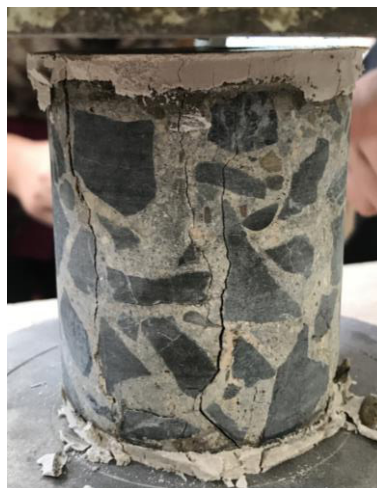
Figure 3.1-1 - Concrete core from girder (MP-2) after compression test
