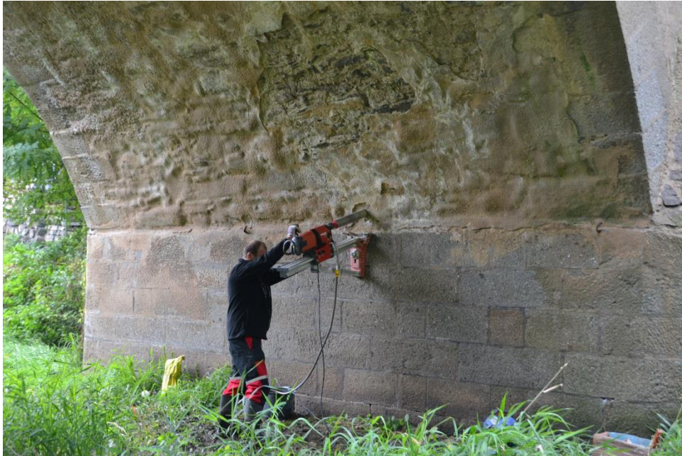
Fig. 32 Taking of specimens from the arch springing at the abutment 1
