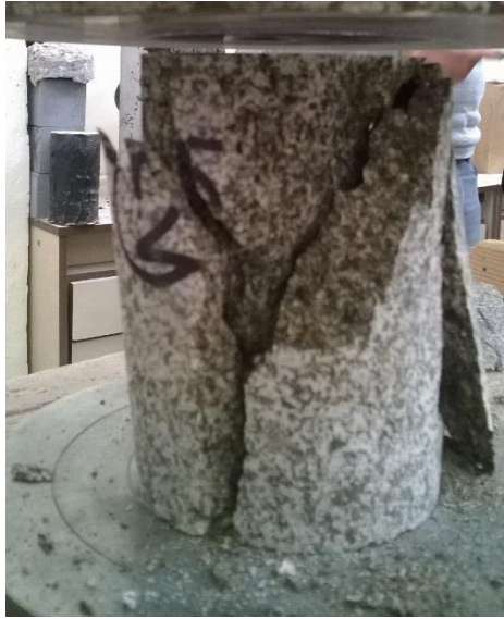
Fig. 36 Specimen no. 2 during loading test
