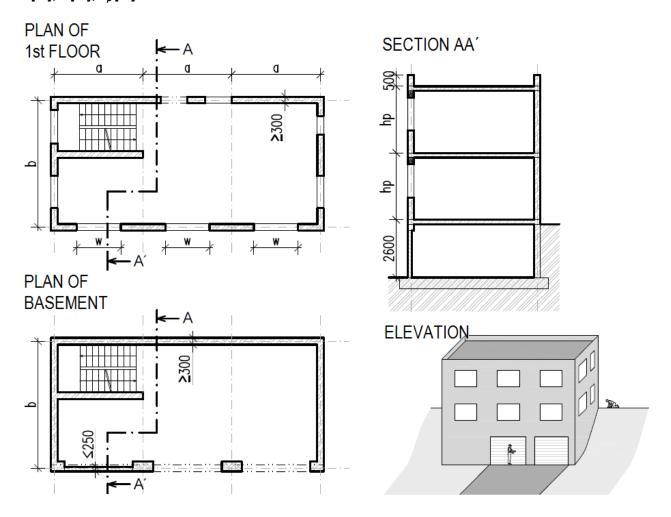
For the pillars in the basement, use solid brick (290 x 140 x 65 mm) of strength category P15 and cement mortar of strength category M5. One of the pillar dimensions is 450 mm, the second dimension will be designed. For the basement walls, use Porotherm masonry of thickness 400 mm. For load-bearing walls of  $1^{st}$  and  $2^{nd}$  floor, the Porotherm wall thickness is 300 mm. For non-load bearing Porotherm walls, the wall thickness is 150 mm.
