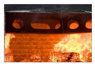
Slab and cellular beams during the fire test
