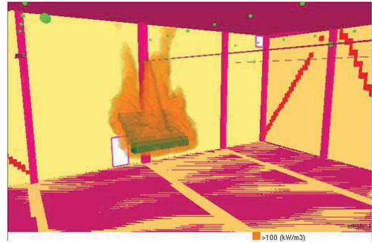
Fig. 10.33 The geometrical model of the volleyball hall Fig. 10.34 The stand fire in the volleyball hall
