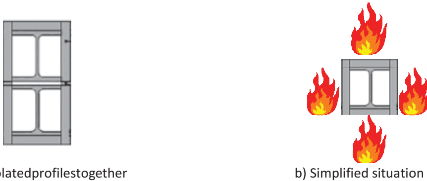
a) Two isolated profile together b) Simplified situation Fig. 24.5 Representation of the fire action to the columns –Case B
