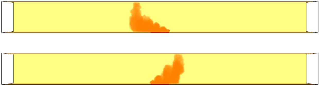
Figure 9.1: Snapshots from the sample case pressure_boundary showing a fire in a tunnel leaning left, then right, due to a positive, then negative, pressure imposed at the right portal.
