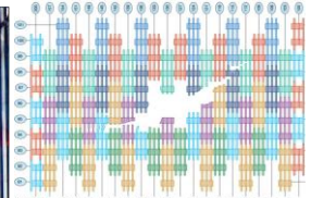
Impact damage to ext. columns on N face of WTC 1
