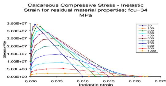
Figure 2 Stress-Strain Curve of Concrete in Compression
