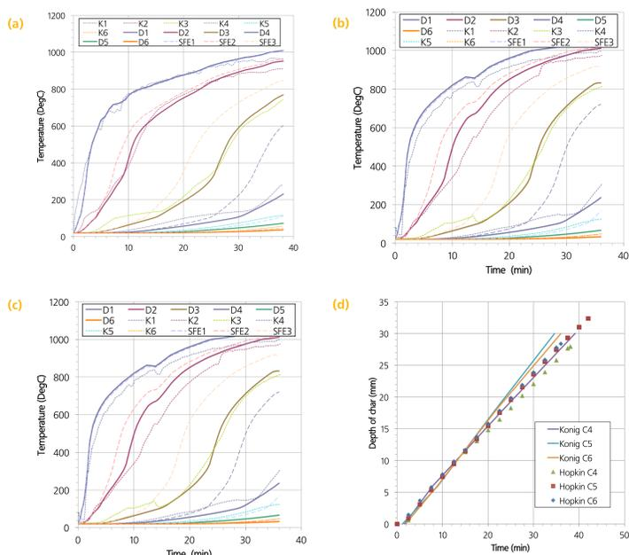
Fig. 1 (a-c) Temperature development, comparison of MCM (D), Konig (K) and EN 1995-1-2 (SFE) simulations/experiments; (d) Transient depth of char- simulation (Hopkin) versus experiment (Konig)
