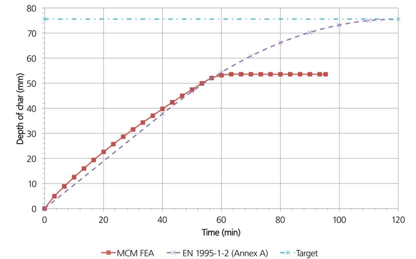
Fig. 2 Comparison of FEA, MCM and EN 1995-1-2 calculation of depth of char
