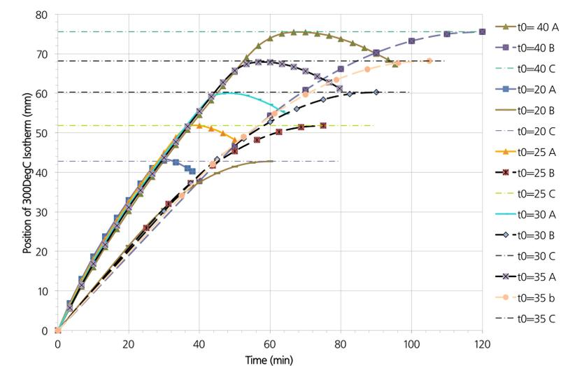
Fig. 3 Position of 300°C isotherm using modified  $k_{qtd,mod}$  (A) and EN 1995-1-2 Annex A (B). Target depth of char shown as (C).
