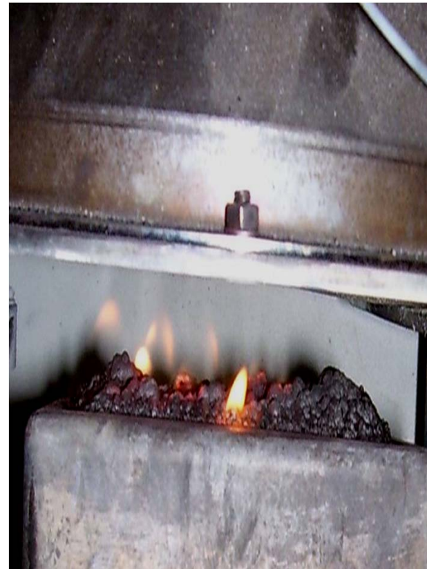
'Zero Flame' treated Pine exposed at Heat flux 65 kW/m 2
