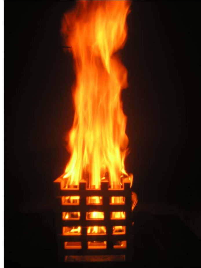
Untreated pine crib at 550 sec. into the test.
