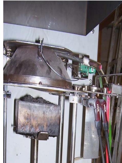
'Zero Flame' treated Pine exposed at Heat flux 35\text{ kW/m}^2
