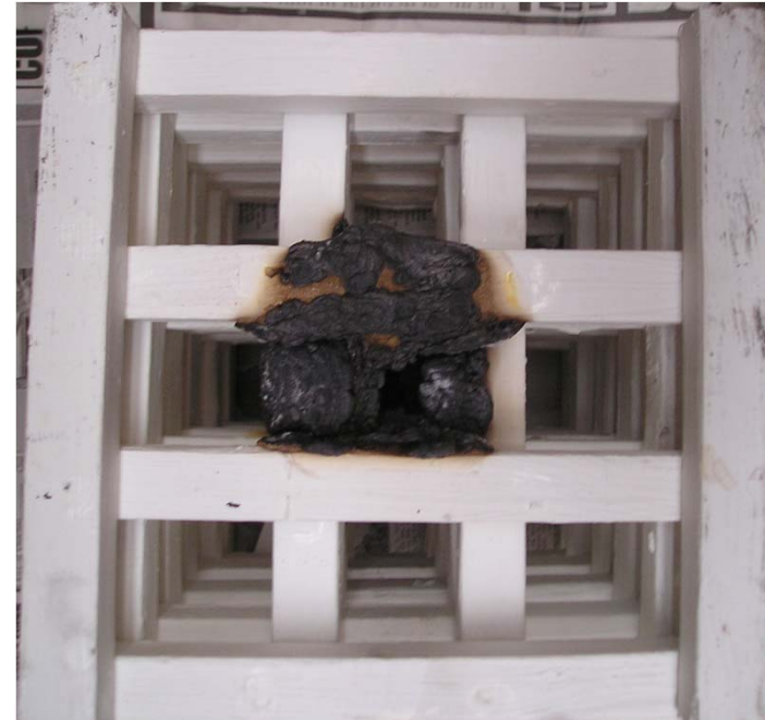
100% treated pine crib (used 20g of ethanol as ignition source) in the end of experimental process.
