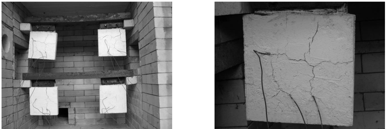
Fig. 4 Reaction of spray coating in fire
