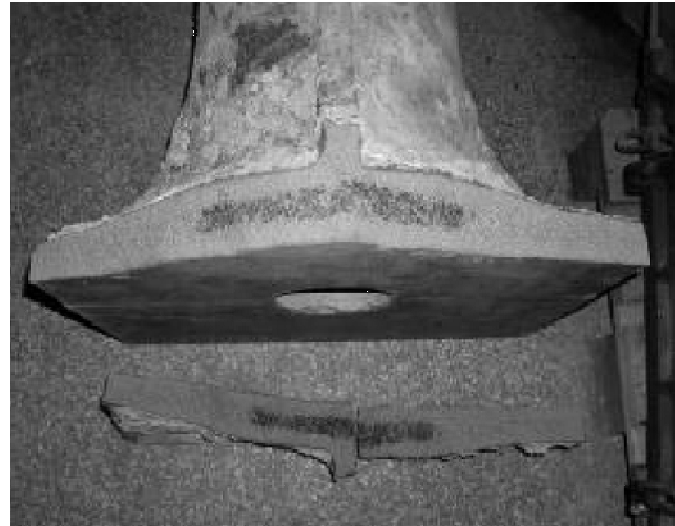
Fig. 6 Failure of base plate during the column test at elevated temperature
