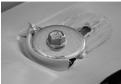
Fig. 6. The collapse mode of connection from the set B, temperature 200°C
