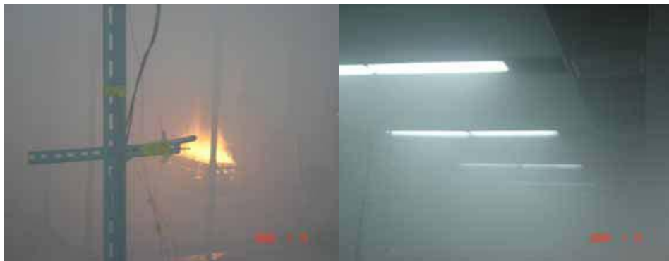
Figure.3. smoke movement in concourse during hot smoke test (fire source at the center of the concourse)
