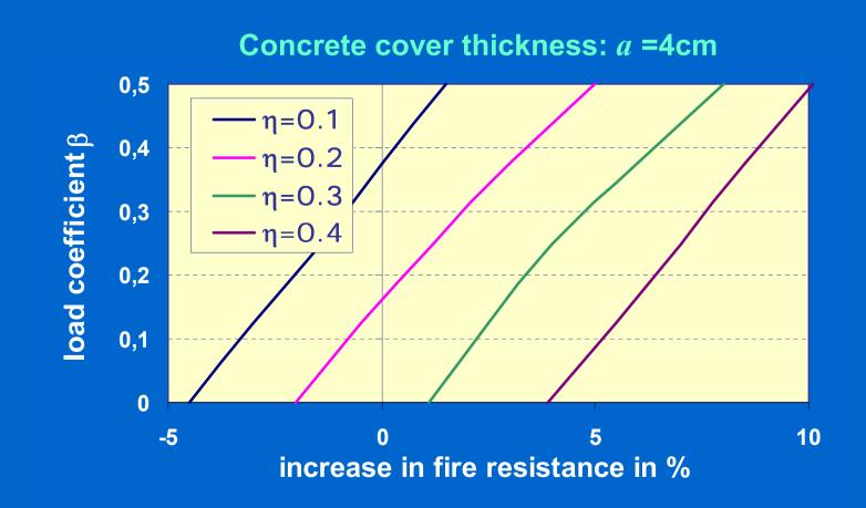
case when the column is centrically loaded ( $\beta$ =0). When the bending moment is increased and the axial force is decreased the positive effect is more expressive.
