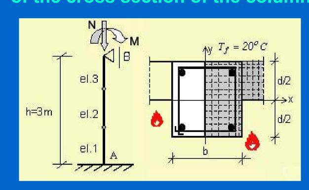
Isotherms in the cross section of column 30\*30cm, as a part of a wall that separates the fire compartment
