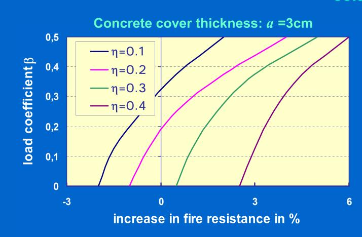
2/ For optimally loaded columns (η≤3) the concrete cover 3/ The effect of steel ratio increasing is positive. That is not a thickness has a positive effect on fire resistance increasing, but not more than 5% for columns with small dimensions, and up to 10% for larger columns.
