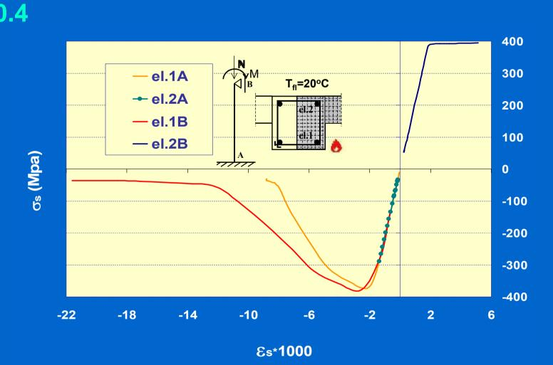
Increase in fire resistance of eccentrically loaded columns when the concrete cover thickness is increased, reference column:a=2cm
